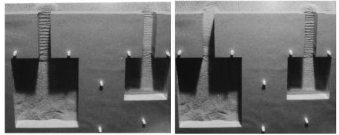
(a) Resonance for large resonator (170 Hz).
