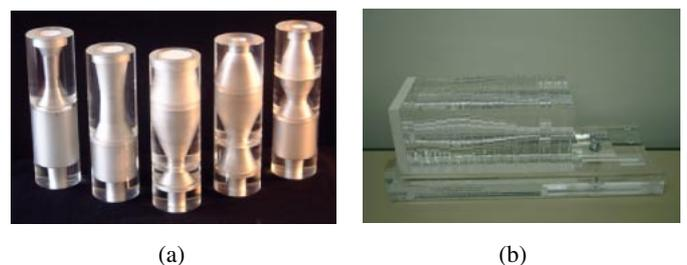
**Fig. 8** Arai’s models of human vocal tract: (a) cylinder-type models (from left, /i/, /e/, /a/, /o/ and /u/); and (b) plate-type model.
