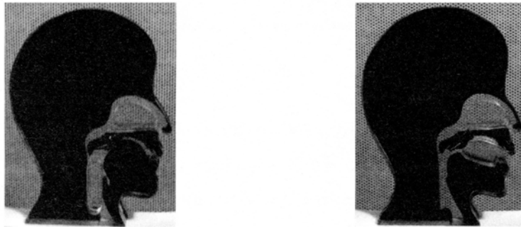
Fig. 2. Physical models of the human vocal tract with the nasal cavity for [i] (left) and [a] (right).
